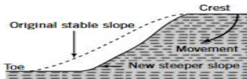
(a) Steepening of slope by erosion
