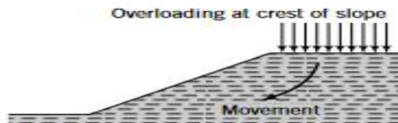
(f) Overloading at the crest of the slope
