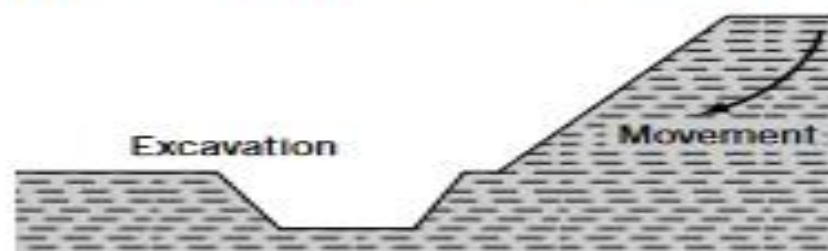
(g) Excavation at toe of the slope
