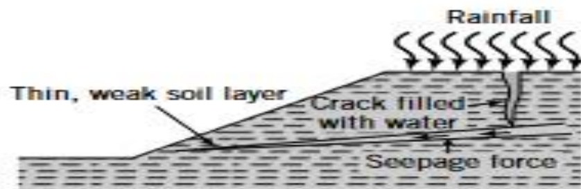
(c) Rainfall fills crack and introduces seepage forces in the thin, weak soil layer
